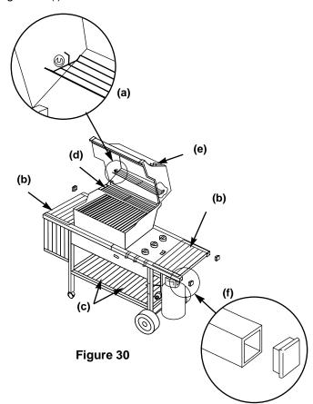
**△CAUTION:** To keep the barbecue stationary, the tabs on the locking casters should be in the down position.
